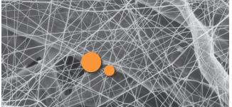
The fibers in the Thermo King filter media have submicron diameter and small interfiber spaces, which result in more contaminant being captured on the surface of the media and lower restriction.
