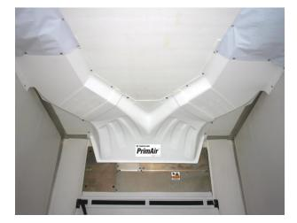
The PrimAir Split Air Chute System is designed to provide uniform temperature throughout the entire trailer. The unique diverter evenly distributes air to each side chute, which then guides the air to the rear of the trailer.
